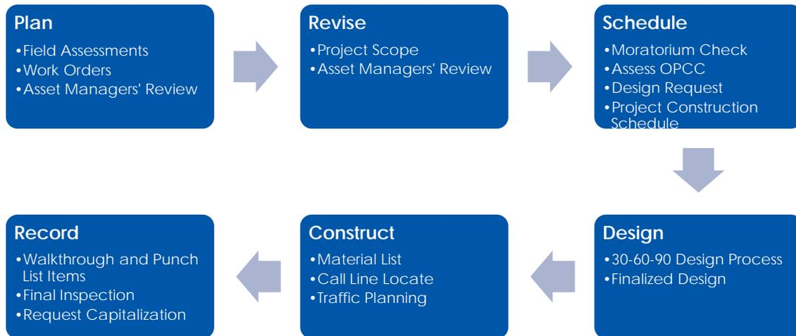
Checking street moratorium and obtaining right of way – or ROW – permits are important steps in planning wastewater construction projects. City ordinance requires every party, external or internal, to apply for a ROW permit if they plan to engage in construction, excavation, or occupy a work area within or upon any right of way.
